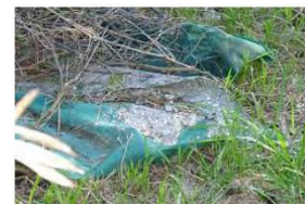
Figure 3 Visible amount of AF on from high-pressure cleaning of an asbestos cement roof.
